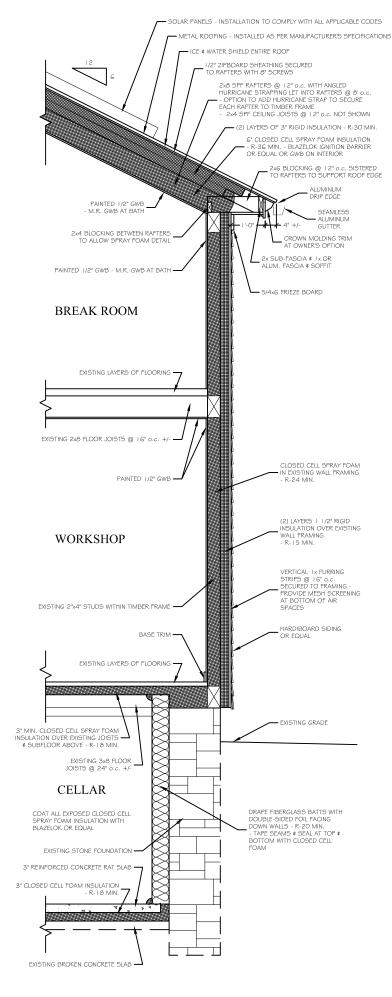
2) DETAILED WALL SECTION SCALE: 3/4" =1'-0"
